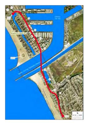
The sewer will originate at the Venice Pump Plant located on Hurricane Street and cross Grand Canal, travel east to Marquesas Way, then south along Via Marina crossing the Marina del Rey and Ballona Creek Channels to meet an existing Coastal Interceptor Sewer junction structure on Vista del Mar near Waterview Street.
